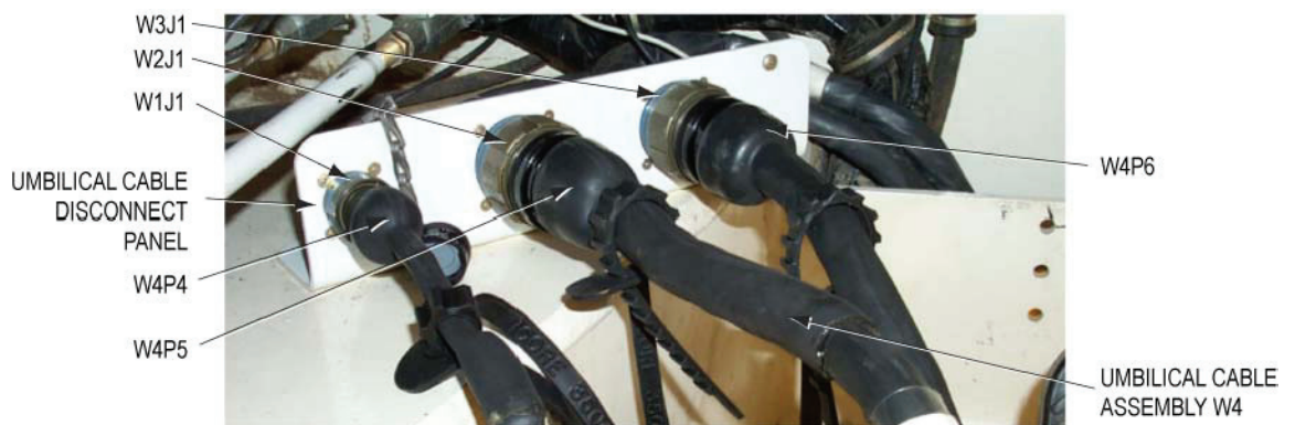
Figure 13. Umbilical Cable Assembly W4 Connection to Umbilical Cable Disconnect Bracket
