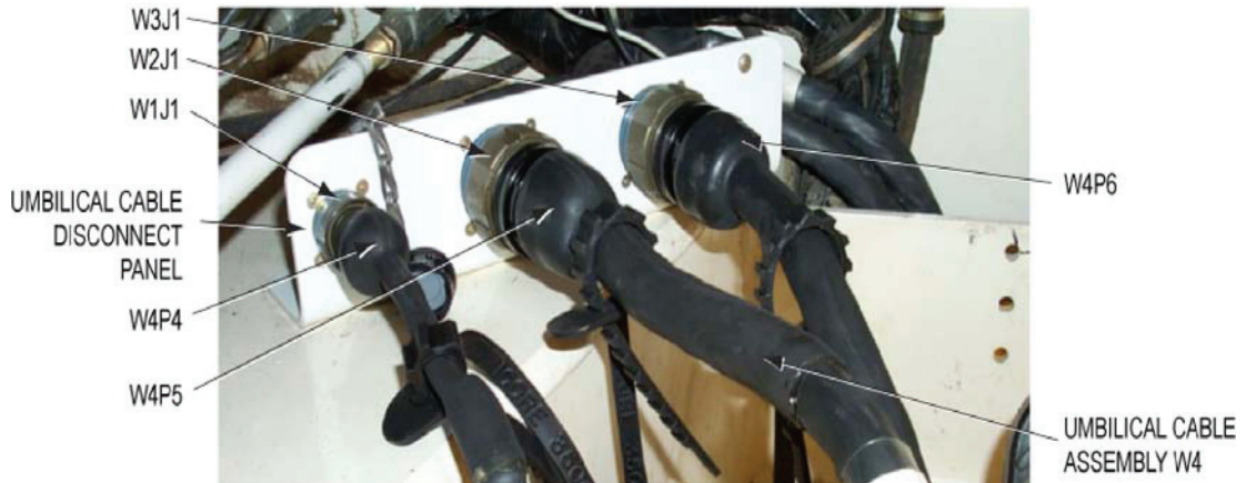
Figure 1. Umbilical Cable Assembly W4 Connection to Umbilical Cable Disconnect Bracket
