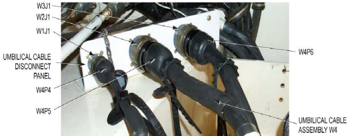
Figure 24. Umbilical Cable Assembly W4 Connection to Umbilical Cable Disconnect Bracket
